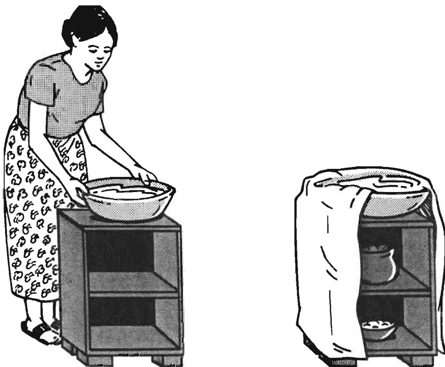
Fig. 10. A cooling cupboard.
